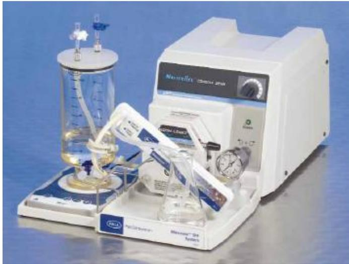
*The Minimate TFF system includes all the hardware, tubing and fittings needed to get your TFF process up and running quickly. Simply connect the Minimate TFF capsule for efficient concentration or diafiltration of your sample.*
